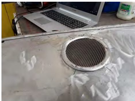
New grille fitted to the towing hatch of Cardiff 262. Hatch being paint stripped, to be followed by primer [Keith Walker]
