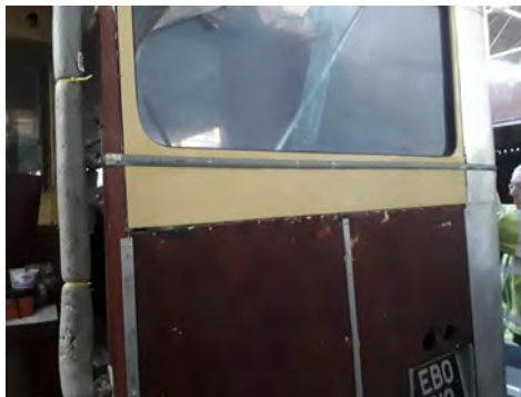
Rear beading fitted to Cardiff 262. [Keith Walker]
