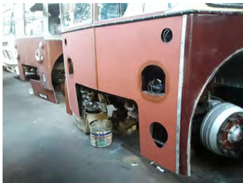
New front panels and beading fitted to the front of Cardiff 262. [Keith Walker]
