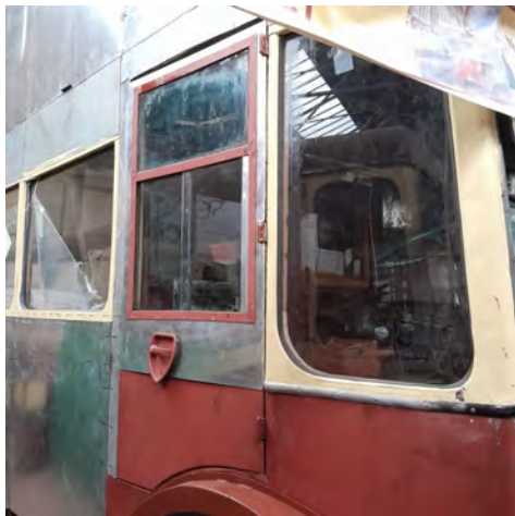
Driver's door window frame reassembled and three panes of glass fitted. [Keith Walker]
