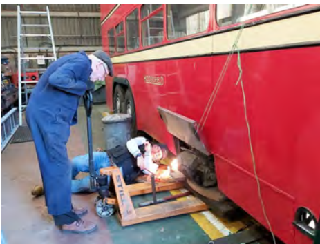
Mike Hurst and Tony Walsh succeed in removing Huddersfield 619's compressor. The trolleybus was reluctant to let it go!
